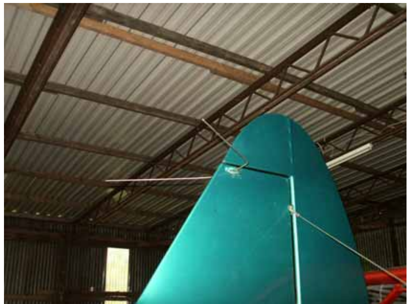
An Example of VOR Aerial
