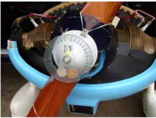
couple of pounds. In use the device is fixed to the prop with rubber bands and the engine turned to TDC and the protractor set at zero. It is then easy to turn the prop the number of degrees called for by the engine manual. If you have a specialised implement, please let the editor have details so that it can be passed on to other Strut members.
