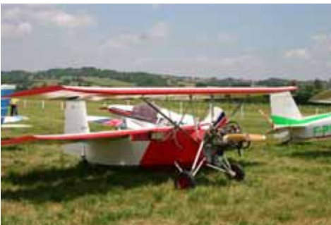
The Mignet Pou de Ciel concept is still popular in France. This Pou derivative was a single seater with VW power.
