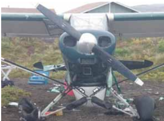
Ripped Tyres and bent Tailplane Leading Edge
