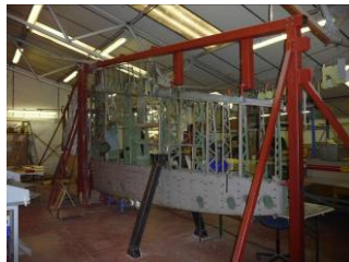
Spitfire wing in jig and stripped down fuselage
