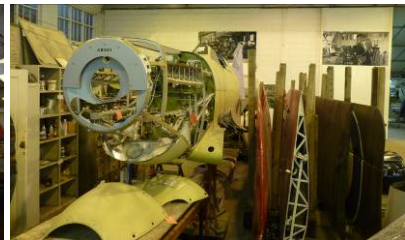
Spitfire wing in jig and stripped down fuselage
