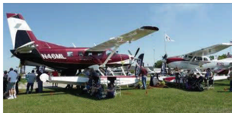
Aerocet / Kodiak - 162KTAS at 10,000' from 750shp PT6A-34 6650 series composite floats
