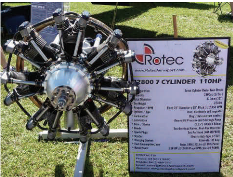
Rotec 7 cyl 110 hp and 9 cylinder 150 hp both at 2450rpm
