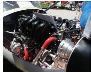
Viking, 130hp $11,995 based I believe on Honda. Fitted to— Zenith, Sonex, Kitfox, Just Aircraft, Van's and Gyro's (their apostrophes). _____ This one on a SeaRey
