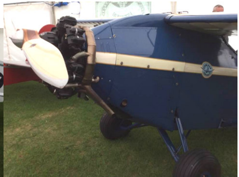
Comper Swift with very coarse pitch prop.
