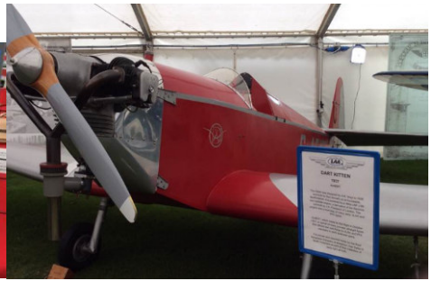
Dart Kitten designed in 1936 by A R Weyl and built in Dunstable by Dart Aircraft with a 36 hp JAP two cyl. engine
