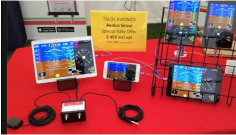
Talos from Greece runs all these displays. £499. GPS antenna on left, OAT on right, magnetic compass & attitude sensors built in, static and pitot ports.
