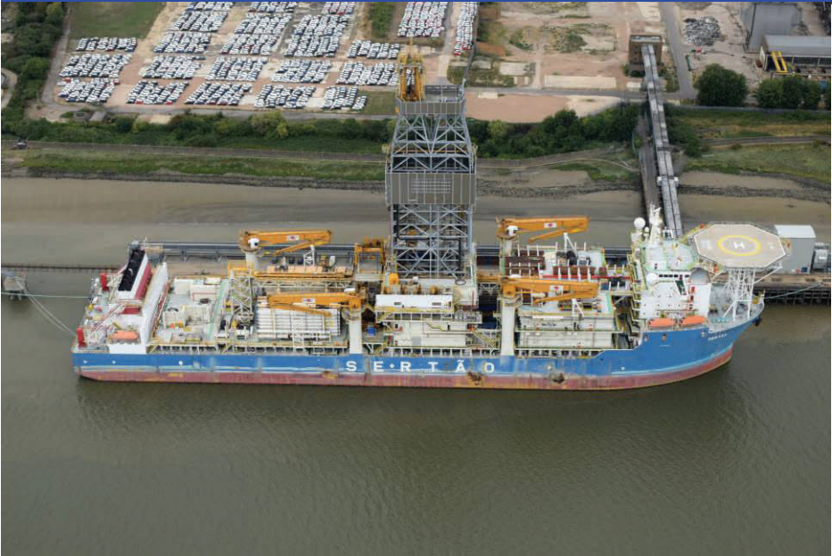
SERTAO Drill Ship, Gross tonnage 60316, 227.8m x 42m. The ship can drill to 40,000' in 10,000' of water. marinetraffic.com
