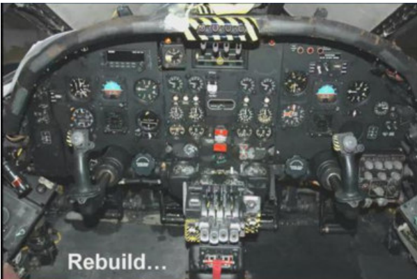
One of the early test pilots, Roland Falk suggested fitting a fighter style control column instead of the more common bomber style yoke.
