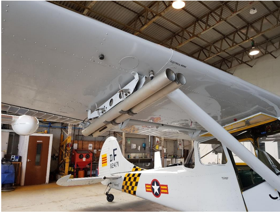
Starboard pair of fully functional rocket launchers
