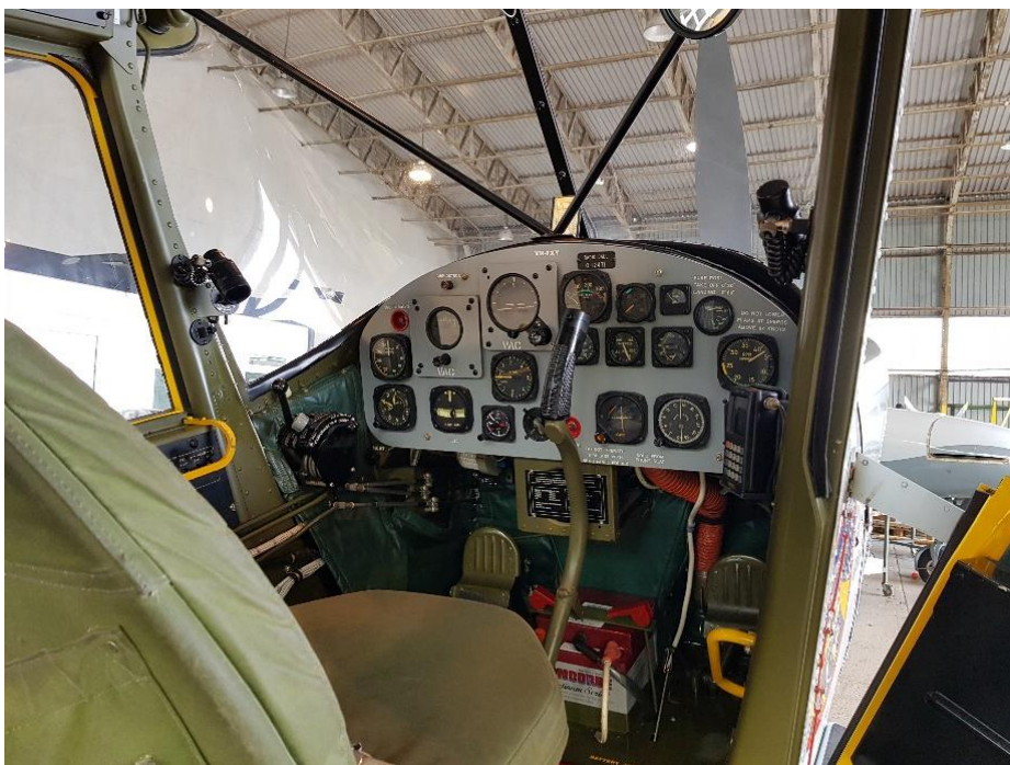
Utility panel for the Pilot in Command
