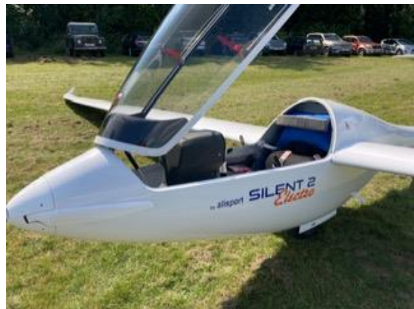
Electric self-sustaining, the battery lasts about 30 mins gently cruising and about half that, climbing.
