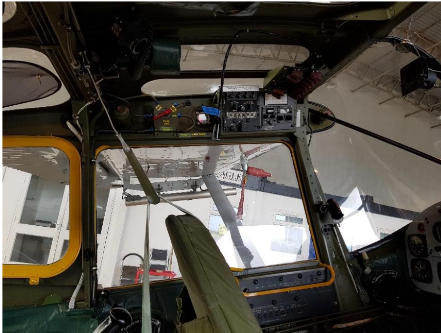
Overhead radios, fuel selector and breakers
