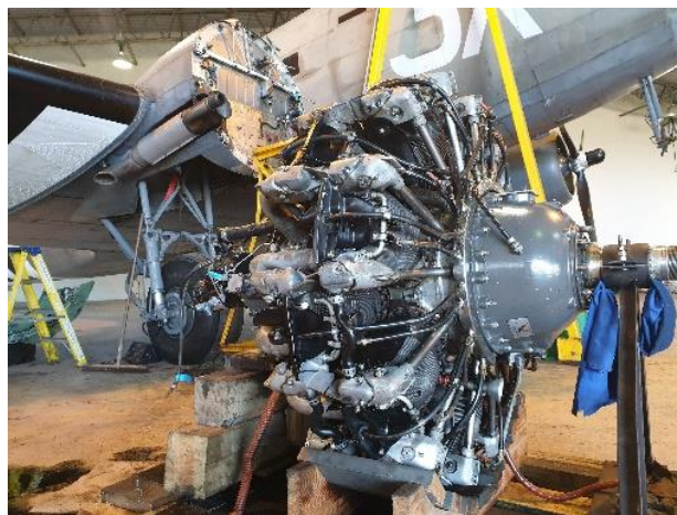
DC3 power plant change
