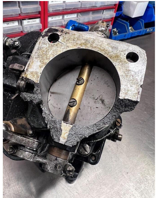
Damaged mounting flange on original
